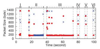
Fig. 3. The IPSec packets of six Wi-Fi calling events over time (×: uplink packets; ■: downlink packets; I/VI: Activating/Deactivating Wi-Fi calling; II/III: Receiving/Dialing a call; IV/V: Sending/Receiving a text).
